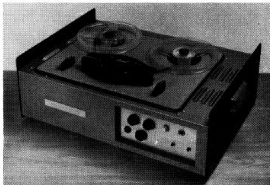
Left — the simple yet ultra-reliable unit produced for continuous music applications Below is the editing console for producing special tapes for The British Library of Tape Recordings for Hospital Patients. These are made on 16mm tapes at a speed of 2 inches per second
